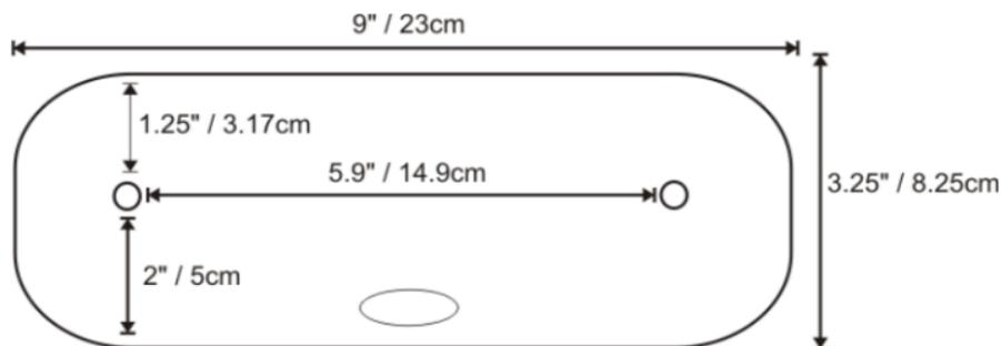
Place the charger on a horizontal, hard surface or fasten securely to a wall using the mounting holes. Mounting hardware is not supplied by Honeywell.
