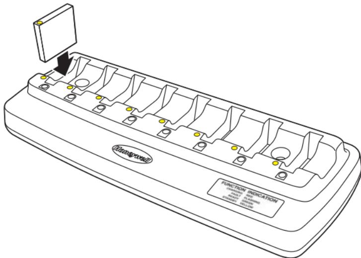
It is important that batteries are inserted into the charging pocket correctly. Inserting the battery incorrectly could result in damage to the battery or the charger. Do not “slam” or slide the battery into the pocket. This could damage the charger.
