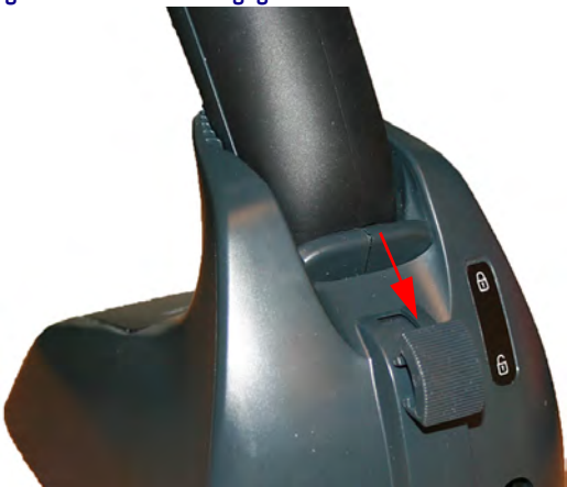
Figure 1. Lock lever disengaged
